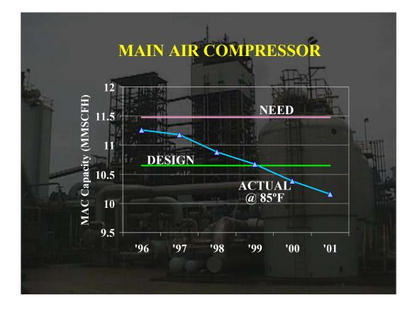
Polk's oxygen plant requires about  $11\frac{1}{2}$  MMSCFH of air to produce enough oxygen for full load operation on a variety of fuels over the normal ambient temperature range and to simultaneously reprocess enough fines to generate a slag product suitable for cement industry. This is about  $8\frac{1}{2}\%$  more than design.
