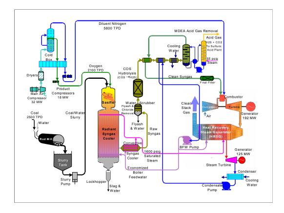
This is a schematic flow diagram of the Polk IGCC system. A description of the process can be found in Tampa Electric's 1999 Gasification Technologies Conference paper.
