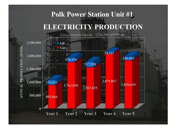
This is an overview of Polk's five years of commercial operation. Year 4 was our best to date, with a gasifier capacity factor of 75%. Last year's gasifier capacity factor was only 66%, but production from distillate fuel brought the overall capacity factor up to 71.8%.
