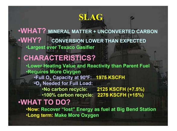
Slag is the noncombustible mineral matter contained in coal plus any of the coal's carbon which was not converted to syngas in the gasification process. In previous papers at this conference, we have discussed the fact that there is approximately twice as much unconverted carbon from Polk's gasifier as initially expected. This unconverted carbon makes Polk's slag unsuitable for all known applications unless it is further processed.
