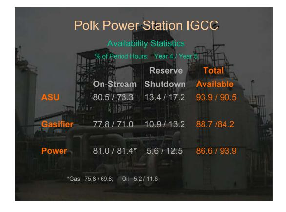
The term "Reserve Shutdown" is equivalent to the GTC's category "Product Not Needed". For the ASU and Power Block, this is straightforward. For the Gasification Plant, this reflects the percentage of the time when the gasifier was intentionally not operated for economic reasons, or when either the power block or the oxygen plant were unavailable.
